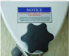
10) Once the machine has reached operating speed, look at the digital pad pressure meter located on the top of the motor cover. There are 3 light colors which will help you determine optimal pad pressure for operating the machine. RED LIGHT(S): If one or both red lights are illuminated, stop the machine and turn the pad pressure
