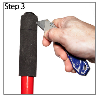
Step 3 Cut from the top down to where you made your mark at 1 1/2".
