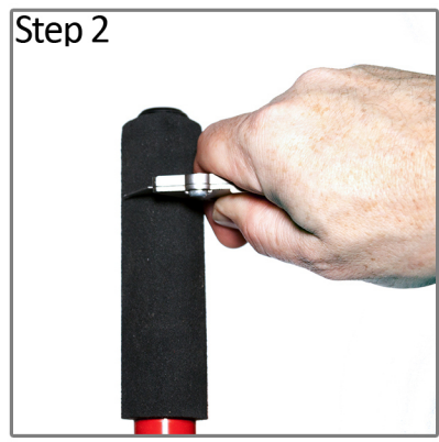
Step 2 Cut Horizontally all the way around the handle at the 1 1/2" mark.
