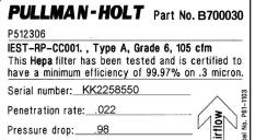
Each Pullman-Holt HEPA filter is tested and certified to provide a minimum efficiency of 99.97% at .3 microns. based on IEST-RP-CC001 test requirements.
