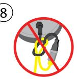
Do not tie extension cord and power cord together. Doing so will result in damage to both cords and will not be covered under warranty.
