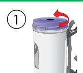
Unscrew the cap on the top of the vacuum unit.
