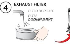
For backpack models (with an exposed exhaust filter) rinse, air dry and return the foam filter/diffuser to the bottom of the vacuum below the motor. This should be done weekly or as neccessary.
