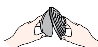
Pull the top piece of the Dome Filter off and remove the foam media. Shake it out, rinse it, and let it air dry thoroughly. HEPA MODELS: For best results replace pleated dome filter every 6 months (or more often if necessary).
