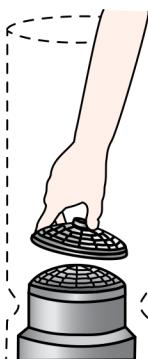
Once a week, or as necessary, clean or replace the Dome Filter. First, remove the Intercept Micro Filter and Cloth Filter. Reach into the vacuum body and twist dome filter from motor.
