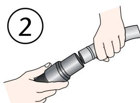
Twist the wand onto the end of the hose.
