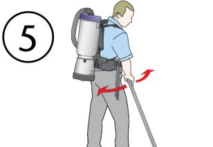
Twisting at the waist, vacuum in a side-to-side motion while walking backward or forward.
