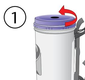
Unscrew the cap on the top of the vacuum unit.
