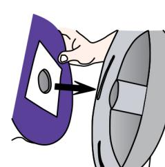
For vacuums with closed top bags, slide the gasket of the filter over the inlet on the inside of the top cap, then replace the cap.
