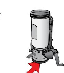
For backpack models (with an exposed exhaust filter) rinse, air dry and return the foam filter/diffuser to the bottom of the vacuum below the motor. This should be done weekly or as necessary.
