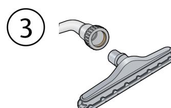
Attach the floor tool to end of wand. Align the brass ring with the indentation on the floor tool to ensure a secure fit.
