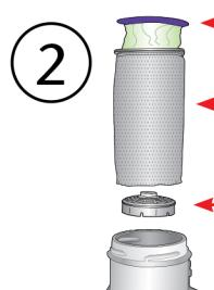
Check to make sure the filters are in place and have not shifted during shipping.
