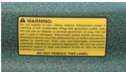
**⚠ WARNING LABELS - Located on back and top. Labels warn operator of safe practices for equipment**
