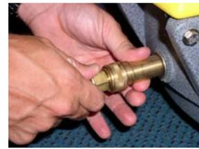
**Step 6** - Connect vacuum hose to recovery tank. (Located on front of machine)
