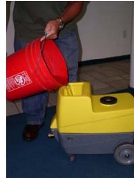
**ATTENTION:** Do not use recovery tank to fill solution tank. Residual dirt or debris will cause damage to solution pump.
