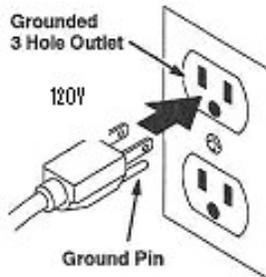
**FOR SAFETY: Do not operate machine unless cord is properly grounded. Do not operate machine with the use of additional extension cords.**
