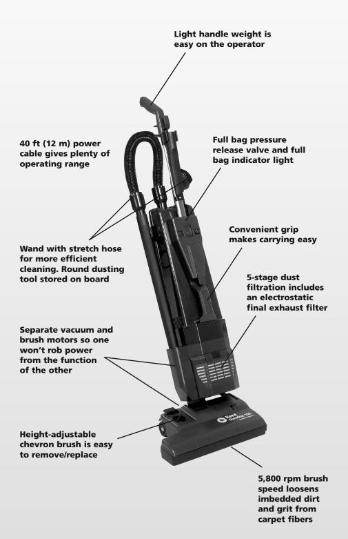
The DuraVac® 152 dual-motor upright carpet vacuum cleans a 13.5 inch (34 cm) path, shaking loose and drawing out imbedded dirt and grit that shorten carpet life.
