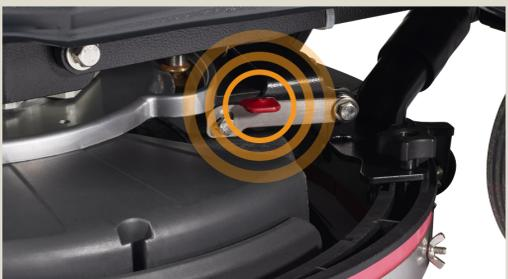
Lift the squeegee up by hand until it locks in up position and turn suction off for double scrubbing. To go back to working mode, use the red lever to release the squeegee. and turn suction on again.
