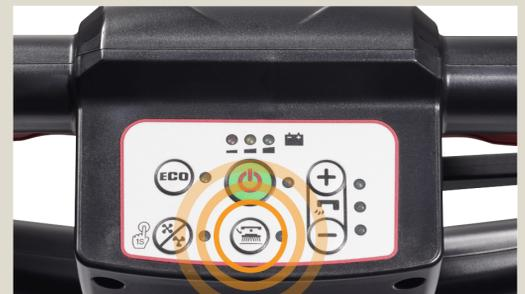
**Daily:** With the machine turned on and the deck lifted, press the click off button to release the brush/ pad holder then clean and inspect before next use.
