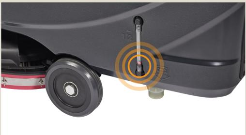
Check the solution level the red ball on the left side of the machine.
