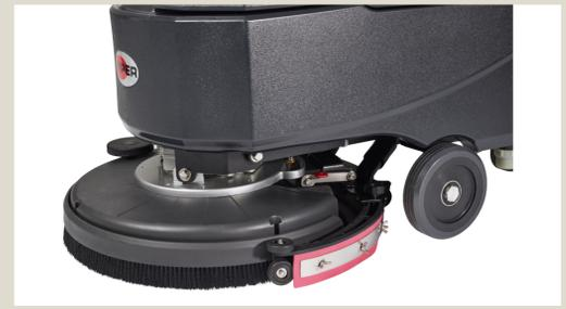
Place the brush or the pad-holder under the deck and Lower the deck or the brush/pad-holder by pressing the pedal
