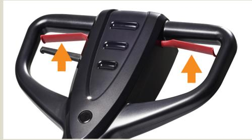
Start cleaning by placing the hands on the safety switches
