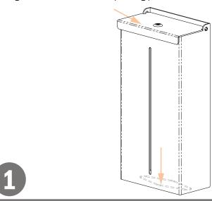
Mount securely to a wall with screws approved and supplied by building maintenance.
