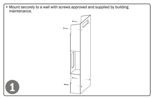
• Dispenser can be mounted to a Bowman Wall or Door Hanger through cutout in back. (See guidelines for door hanger mounting on the hanger instructions.)
