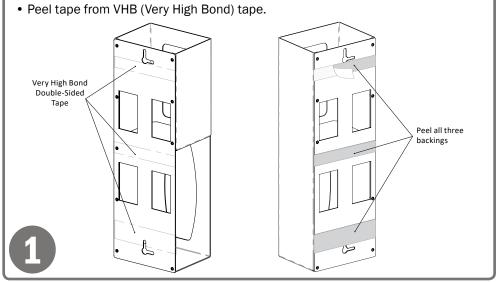
VHB tape is virtually permanent, so it is imortant to align well with the back plate.Line up the back and bottom of the dispenser with the L-shape of the back plate
