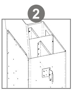
Attach bracket to cart through prethreaded holes on left side of cart as shown.
