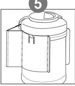
Slide wipe canister into dispenser from top down until pointed notch locks into rib or lip near the lid of the canister.
