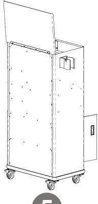
Place left side of bracket over mounting bolts and attach plastic washers and ridged knobs.
