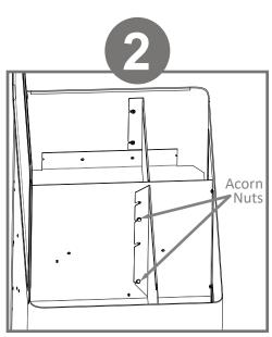
To dispense laundered gowns, loosen the four (4x) acorn nuts holding the divider in position.
