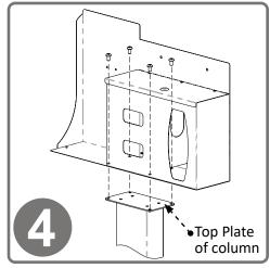
Attach the RS009-0420 Respiratory Hygiene Station to the column using (4x) screws included with stand. One pair of screw holes is located in the hand sanitizer dispener section; the second pair are inside the facemask section and can be accessed with the lid open. Tighten all screws.
