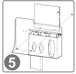
To mount the MP-075 Sign Holder, align the mounting holes of the holder with the holes on the top front of the dispenser. Attach using (2x) barrel screws included with sign holder.
