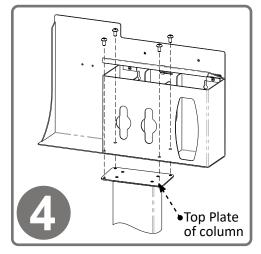
Attach the RS013-0220 Respiratory Hygiene Station to the column using (4x) screws included with stand. Tighten.
