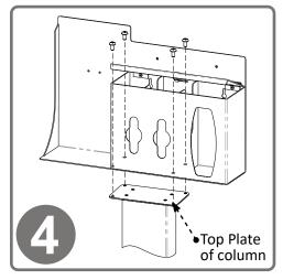
Attach the RS013-0220 Respiratory Hygiene Station to the column using (4x) screws included with stand. Tighten.
