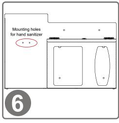
Attach hand sanitizer dispenser using VHB tape or mounting holes provided.
