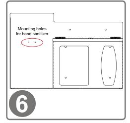
Attach hand sanitizer dispenser using VHB tape or mounting holes provided.
