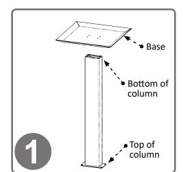
To secure base to column, turn column upside down (with top plate down) and place base inverted, as shown, on column.
