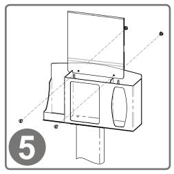
To mount the MP-075 Sign Holder, sandwich the holder over the top edge of the dispenser, lining up holes. With a flathead screwdriver, attach using (2x) barrel screws included with sign holder.
