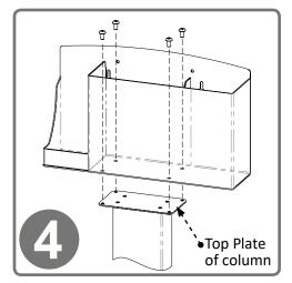
Attach the RS001-0223 Respiratory Hygiene Station to the column using (4x) screws included with stand. Tighten.
