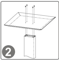
Use Phillips screwdriver to secure base to column with (4x) screws (10-32 x 5/16").
