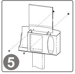
To mount the MP-075 Sign Holder, align the holes of the holder with the holes of the dispenser. With a flathead screwdriver, attach using (2x) barrel screws included with sign holder.
