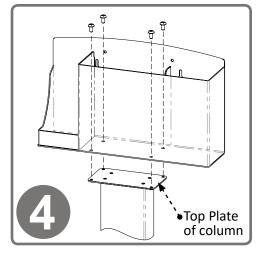
Attach the RS001-0212 Respiratory Hygiene Station to the column using (4x) screws included with stand. Tighten.
