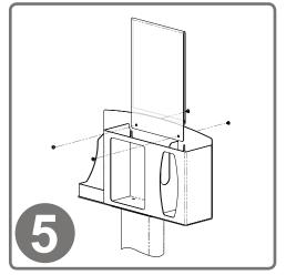
To mount the MP-070 Sign Holder, place the lip of the holder over the front edge of the dispenser, lining up holes. With a flathead screwdriver, attach using (2x) barrel screws included with sign holder.
