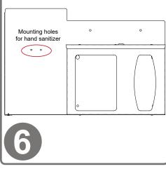
Attach hand sanitizer dispenser using VHB tape or mounting holes provided.
