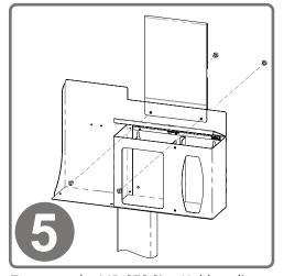
To mount the MP-070 Sign Holder, align the mounting holes of the holder with the holes on the top front of the dispenser. Attach using (2x) barrel screws included with sign holder.
