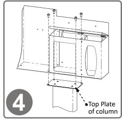
Attach the RS005-0412 Respiratory Hygiene Station to the column using (4x) screws included with stand. One pair of screw holes is located in the hand sanitizer dispener section; the second pair is inside the facemask section and can be accessed with the lid open. Tighten all screws.
