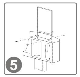
To mount the MP-070 Sign Holder, align the holes of the holder with the holes of the dispenser. With a flathead screwdriver, attach using (2x) barrel screws included with sign holder.
