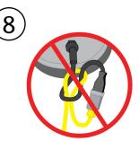
Do not tie extension cord and power cord together. Doing so will result in damage to both cords and will not be covered under warranty.
