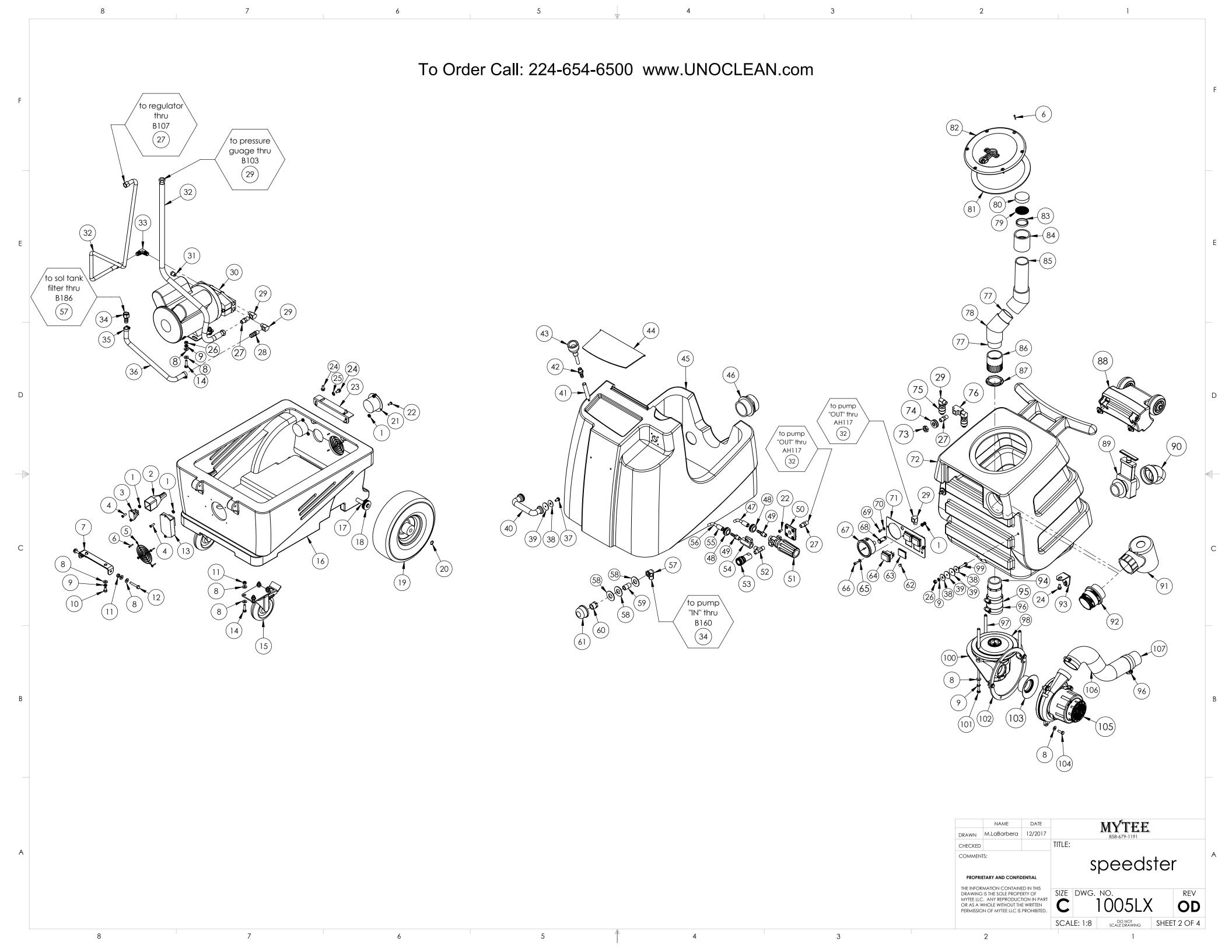
ITEM NO. PART NO. **DESCRIPTION** QTY. H042 c-clip, 12mm, external wheel, 3" 2 H358B H507 axle, 7.94" x .50" dia washer, 1/4" flat, s/s 2 H210 H169 bolt, 1/4-20 x 2", hex head P650 wheel handle, LTD G052 washer, buna 1-1/8" od x 3/16" id H211 washer, 1/4"id x 1"od, flat, s/s 2 H216 nut, lock, 1/4-20, nylon insert, s/s
