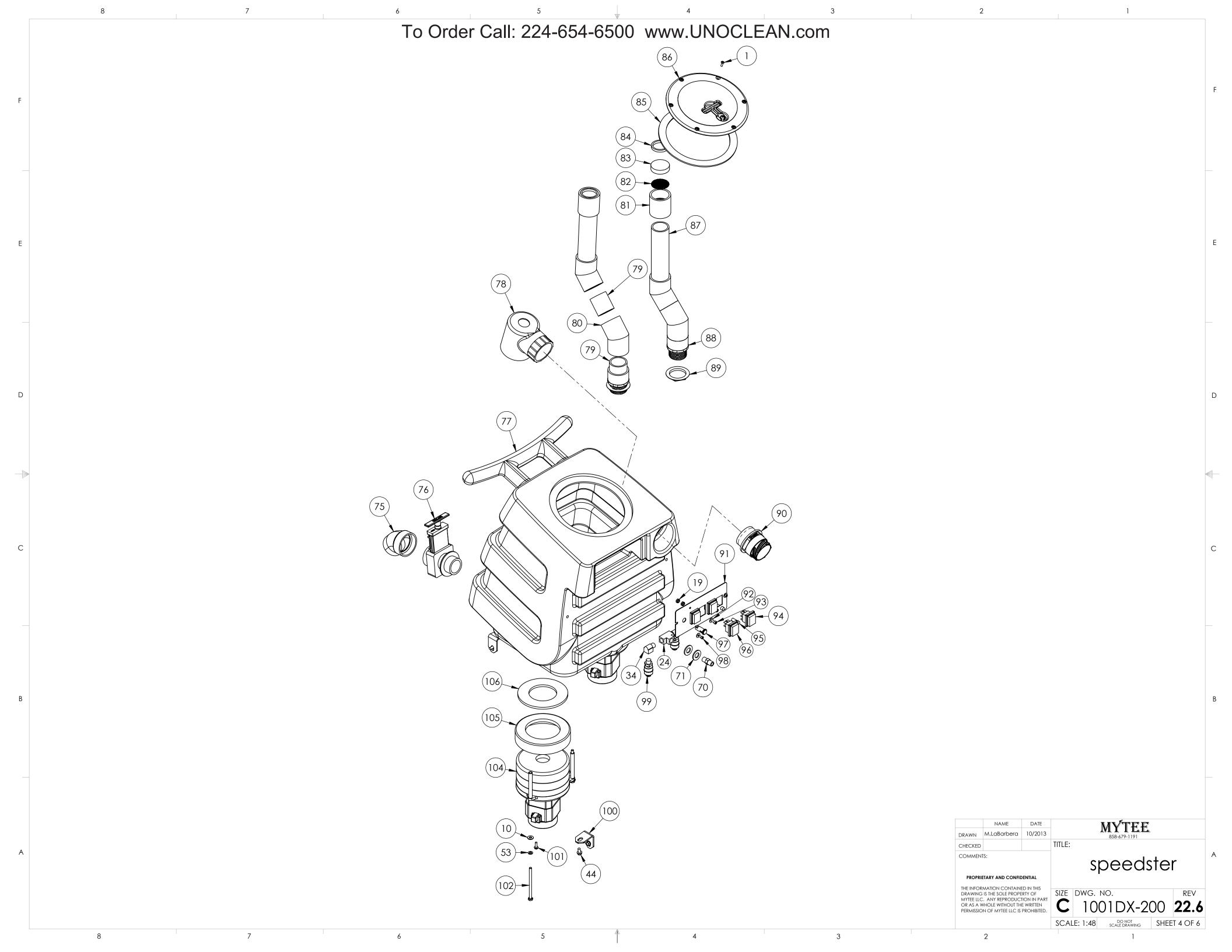
PART NO. DESCRIPTION QTY. B207 elbow, brass, 90 deg, 1/4" fpt x 1/4" fpt AH156 hose, 3/8", (OAL), f x fs, 5400 gray B103 elbow, 90 deg street, 1/4"mpt x 1/4" fpt heater, aluminum cast, single H903A Thermostat, 310°F ± 10°F, Manual, 1/4" E574 E519 heating rod, 1000W, 115V E573 Thermostat, 200°, Auto, 1/4" H274 screw, 6 x 3/16, phil pan head, self-tapping
