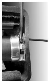
4. Pull out old brush roll from the sweeper. This will release the tension from the belt.
