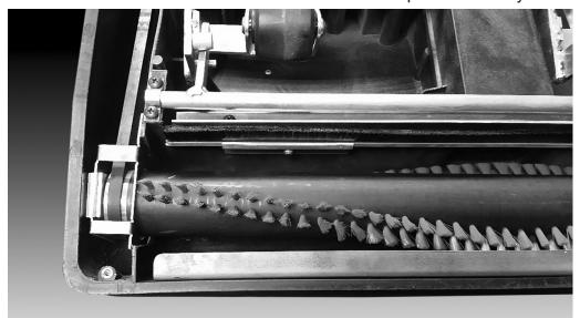
6. Using the 10mm wrench and 4mm Allen wrench, screw in the brush roll with screws and nuts previously used.
