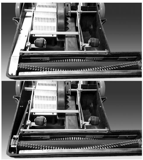
2. Pull down bumper on long end of sweeper to expose screws.
