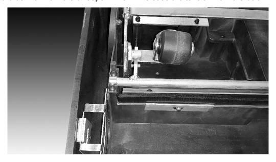
5. Insert the new brush roll. Ensure the belt loops around the grooved end of brush roll and that there is tension in the belt. The brush should be able to spin without any interference.
