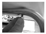
4) Take the nut and place onto the bolt. Finger tighten only.
