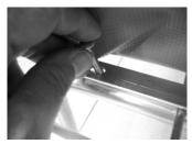
3) Insert the bolt through the basket frame and base until the bolt is visible past the base tube.
