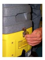
**Step 3 -** Remove recovery tank from solution tank.
