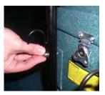
**Step 3 – After** threading by hand, use a 7/16 wrench to tighten (Do not over tighten)
